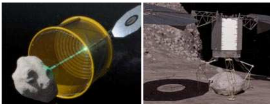
On the left, a notional concept image of ARM robotic capture option A, which would envelop an entire free-flying asteroid. On the right, a notional concept image of ARM robotic capture option B, which would retrieve a boulder from a larger asteroid. Credit: NASA
